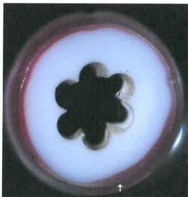
Fig. 3. Red faded core immersed in oil to minimise light scatter. The red colour is not very uniform around the circumference. However, loss of colour from the very outside layer is seen (arrowed).
